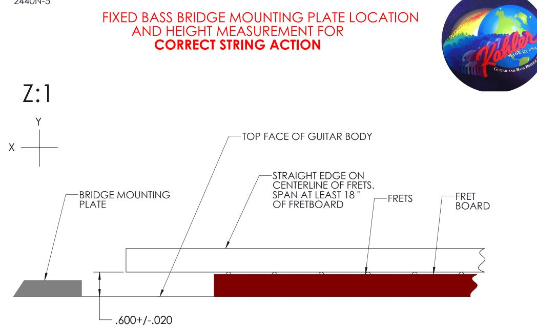
NOMINAL HEIGHT. IF GREATER, ADJUST NECK ANGLE OR ADD SHIMS UNDER BRIDGE PLATE. IF LESS, ADJUST NECK ANGLE OR ROUTE AN INSET.
